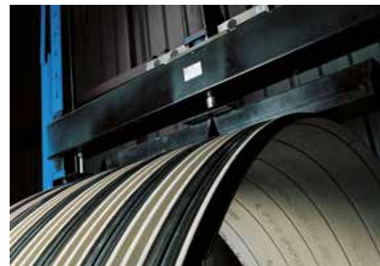
Stiffness testing of SPR™ ST liners
