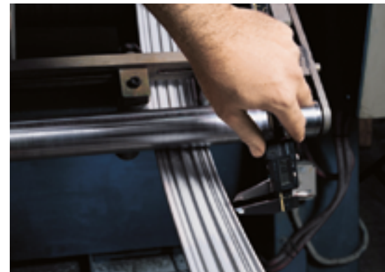
Quality control during the profile extrusion process
